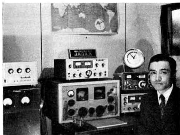
Author of a Japanese 160m manual, Isaji Shima, JA3AA, works a great deal of dx on 1,910kHz using this 1kw set up. (W1BB print)
